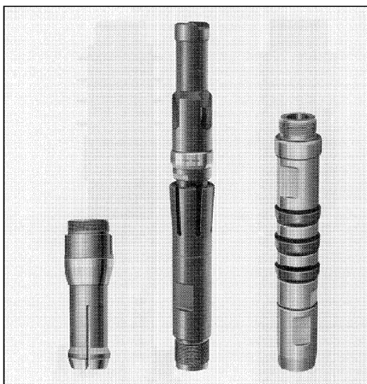
Figure 4. Holddown seal assemblies. The two on the left are mechanical types while the one on the right is a cup type.
