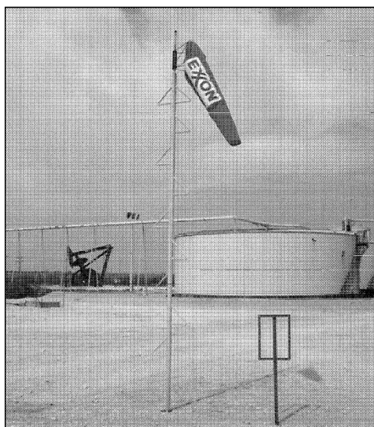
Figure 3. The windsock on the site shows the direction of the wind and whether H 2 S buildup is likely.
